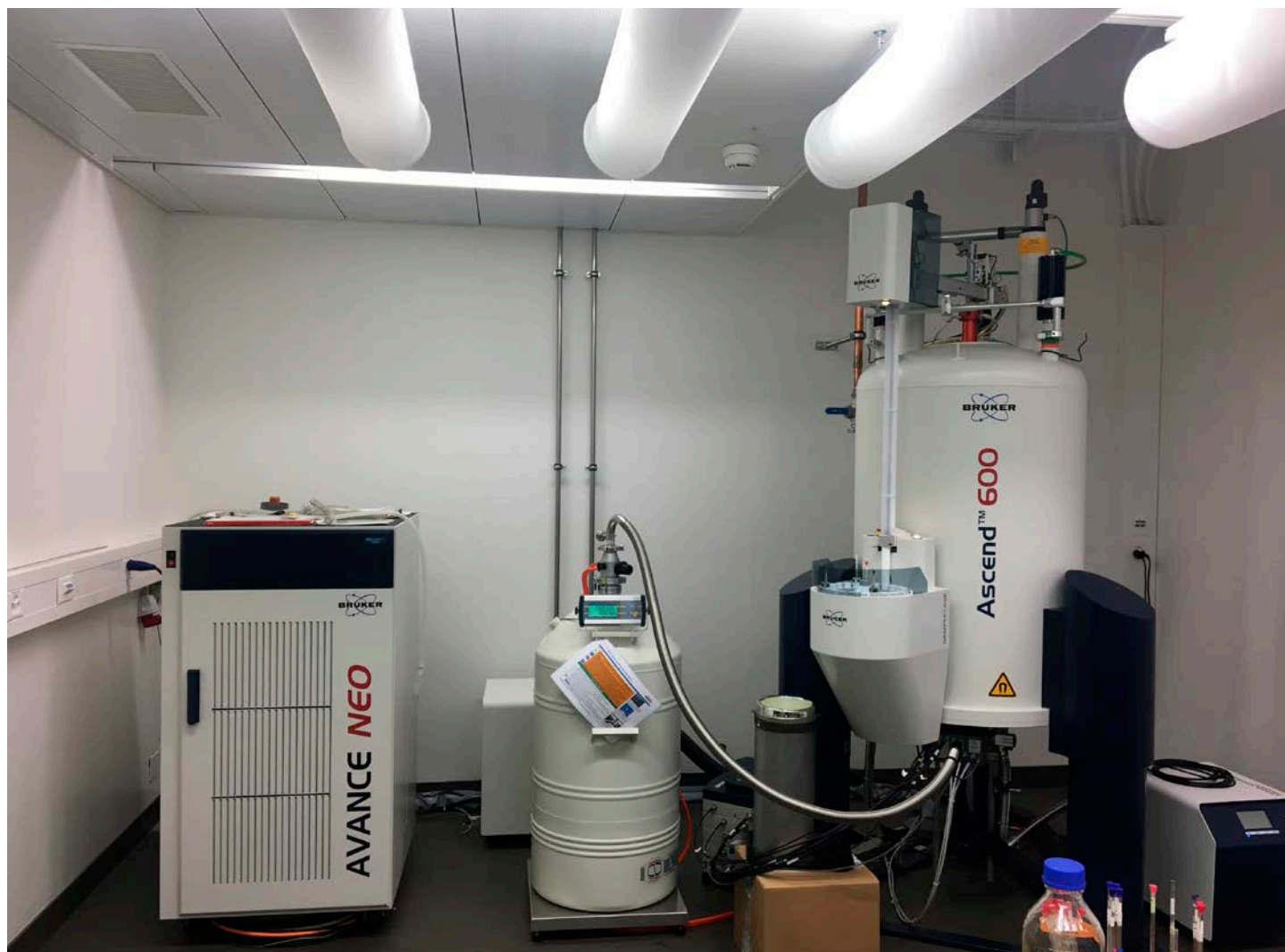
Bruker Avance 600 MHz spectrometer with cryoprobe
